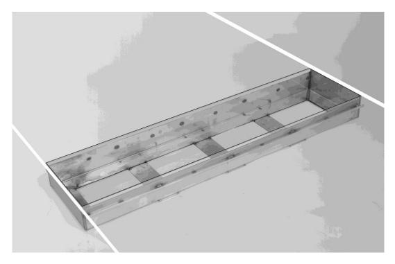
After the cover has been placed in the tray, it should be made sure that the top surface of the cover is levelled with the top surface of the runway. If not the cover feet have to be adjusted.
