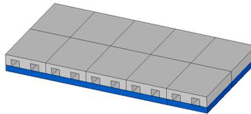
Then position the hollow chamber blocks in the bottom part of the cover.
