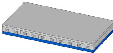
Roll out the anti-wear mat on the hollow chamber blocks and align it centrally.
