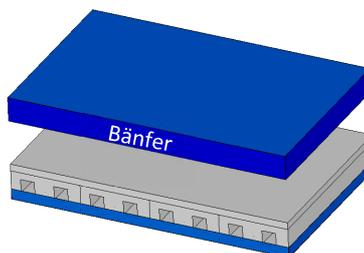
Put the upper part of the cover over the anti-wear mat. Make sure that the ends of the separable zipper match.
