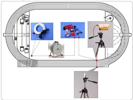
At the start line the starter fires the starting revolver RS-START9, which is connected with the chronometer CHR through the 150 m cable PNB-150. At the finish line the sports photocell FP, which is pointed to the reflector LFP-1, is connected to the chronometer CHR.
