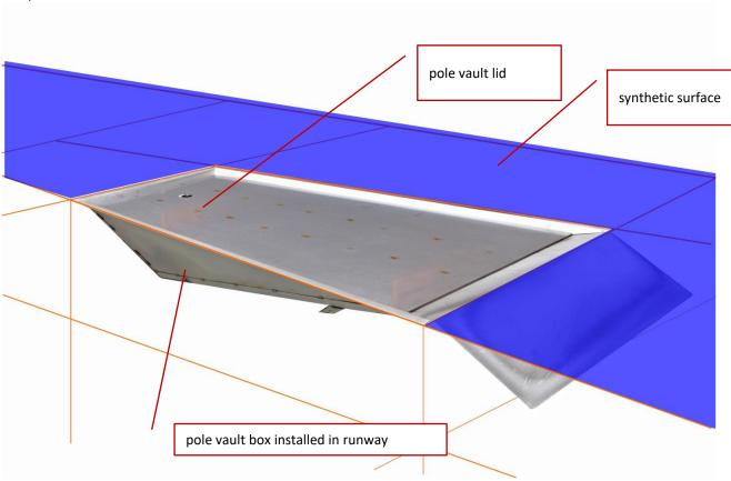
2. A piece of synthetic surface is to fill the space between the lid upper surface and the top of the runway. The lid is designed for the synthetic surface which is approximately 12 mm thick.
