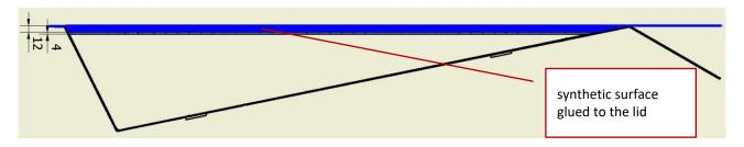
If a synthetic surface piece is to be sprayed or poured on the lid, please place thick foil in the box first, then put the lid into the box and secure the wider edge with adhesive tape. Next install the surface and leave it to dry.
