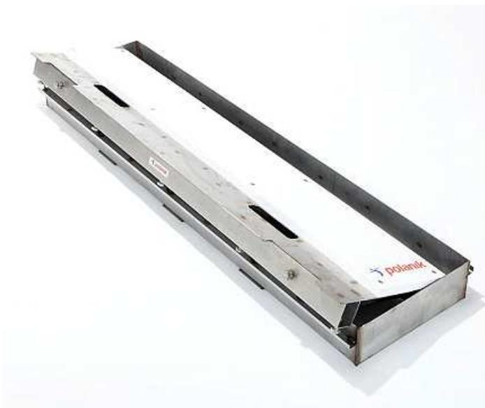
The installation begins with placing the stainless steel base board (item 2) with white take-off board (item 3) in the embedded tray (item 1), so that the square heads of the blocking bolts point the landing pit.
