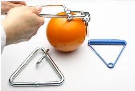
Install the shackle on the swivel, tighten the bolt using the key and the wrench.
