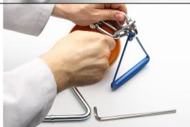
6 Tighten the quick link nut with the wrench.
