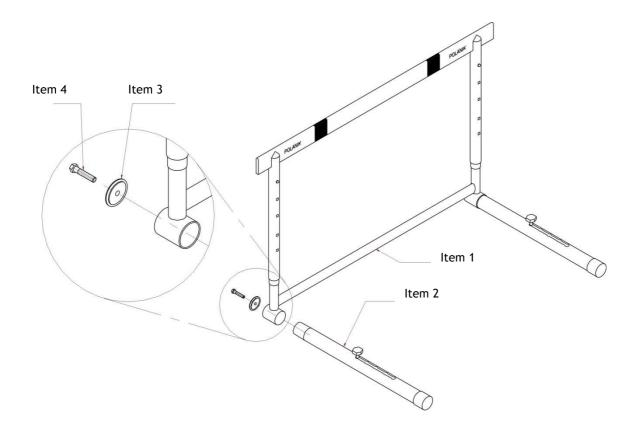
The main goal of the hurdle collapsible construction is to assure easy and cheap transport. Note that once you screw the feet down, the hurdle is practically non-dismountable. Therefore we do not recommend unscrewing the hurdle feet during idle periods. Removing the feet without proper tools can cause serious hurdle damages which Polanik shall not be liable for.
