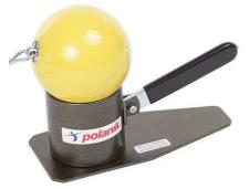
Press the lever all the way down - the steel sleeve (diameter 12 mm) lifts the hammer head (shot put) from the edge. If the hammer head (shot put) stays on the sleeve, it complies with the IAAF rules.
